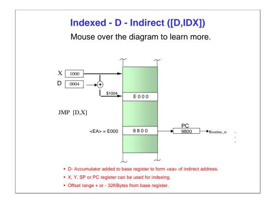
The HCS12 is a very powerful 16 bit microcontroller with a limited number of pointer registers. The limitation in the number of registers is inherited from the HC11 in order to maintain software compatibility. However, the indexed indirect addressing modes gives the HCS12 an unlimited number of memory pointers. This addressing mode in other architectures is sometimes referred to as memory indirect addressing mode.
