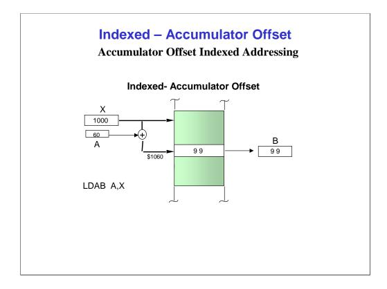
In this indexed addressing mode, the effective address is the sum of the values in the base index register and an unsigned offset in one of the accumulators. The value in the index register itself is not changed. The index register can be X, Y, SP, or PC. The accumulator can be either of the 8-bit accumulators (A or B) or the 16-bit D accumulator. The offset range can be up to + or -32 Kbytes from base register.
