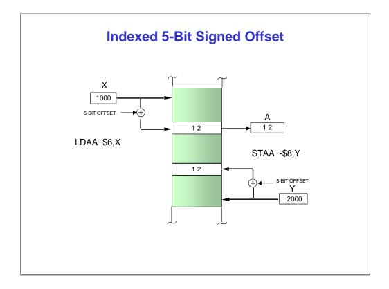
Now, let's look at some examples of the new indexed addressing modes available in the HCS12 instruction set. The first indexed addressing mode shown here uses an efficient short 5-bit signed offset allowing the CPU to access the memory location pointed to by the index register +15 and -16 byte location. The short 5-bit offset is added to the base index register (X, Y, SP, or PC) to form the effective address of memory location that will be affected by the instruction.
