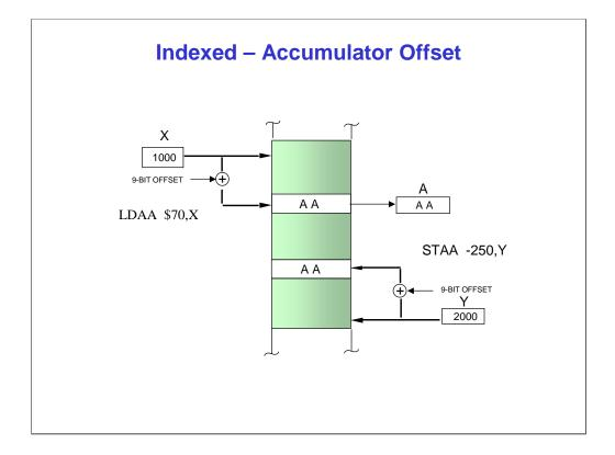
The second indexed addressing mode shown here uses 9-bit signed offset which is added to the index register (X, Y, SP or PC) allowing the CPU to access the memory location pointed to by the index register +255 and -256 byte location.
