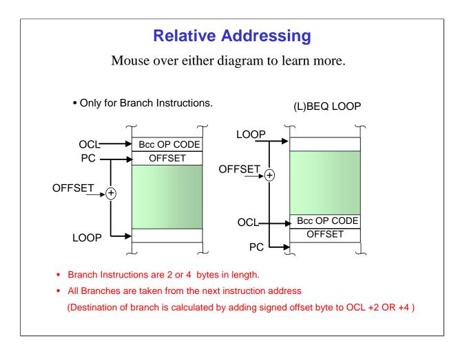
The Program Counter (PC) relative addressing mode is used only by branch instructions. Short and long conditional branch instructions use relative addressing mode exclusively. However, branching versions of bit manipulation instructions (branch if bits set (BRSET) and branch if bits cleared (BRCLR) use multiple addressing modes, including relative mode.
