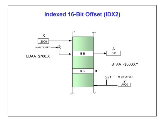
The third indexed addressing mode shown here uses 16-bit signed offset which is added to the index register (X, Y, SP or PC) allowing the CPU to access the memory location pointed to by the index register with an offset of up to +32K and -32K byte locations. This addressing mode, with 16-bit offset, allows the CPU to index to any memory location in the 64K memory map.
