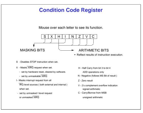
Now, let's look at the condition code register in more detail. Condition Code Flags reflect the results of arithmetic and other operations of the CPU as it performs instructions. These include H, Half Carry; N, Negative; Z, Zero; V, Overflow; and C, Carry/Borrow.
