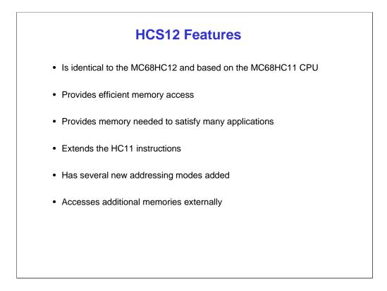
Here is an overview of the HCS12 CPU architecture. The HCS12 CPU is identical to the MC68HC12 and is referred to in most documents as CPU12. Another factor to consider is that CPU12 is upward compatible with the MC68HC11 CPU. The MC68HC11 and the MC68HC12 will be referred to as the HC11 and HC12 respectively in this module.
