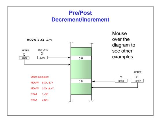
This indexed addressing mode provides four ways to automatically change the value in a base index register as a part of instruction execution. The index register can be incremented or decremented by an integer value either before or after indexing takes place. The base index register may be X, Y, or SP. Note that auto-modify modes would not make sense on PC.
